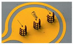
SEM image of 3 cell trapping structures 3D printed onto a measuring electrode. The opening is about 20 µm wide and the struts have a thickness of 1.8 µm.
